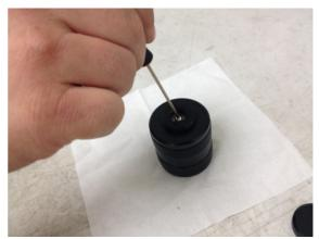
Unscrew the large black handle of the Pressure-Tuner from the brass cylinder. At the outer end of the handle there is a cap which can be unscrewed. Under this cap is a screw that holds the Pressure-Tuner piston.
