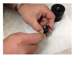
Now you can remove the old O-rings and insert the new ones. After changing the O-rings, maybe you can remove old grease and apply new Teflon grease (part number 0558350) to the O-rings and to the brass cylinder.
