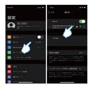
(3) Tapping the SSID will proceed to the screen of entering a password. Enter the initial password "1234567890" set at Vixen's factory. (The name of the SSID and the password are changeable arbitrarily.)
