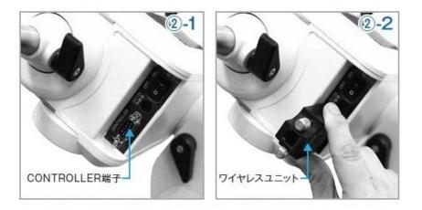
Be sure to attach the Wireless Unit first before connecting the power cord. The Wireless Unit may break if you put on it while the equatorial mount is powered. It avoids a mishap at the setting up in the dark environment where it is hard to check the position of the power switch visibly.
