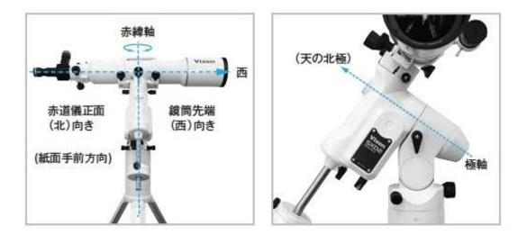
When you fix the position of the optical tube, tighten the RA and DEC clamp levers on the mount. After this, do not touch the clamp levers until you finish your observing.
