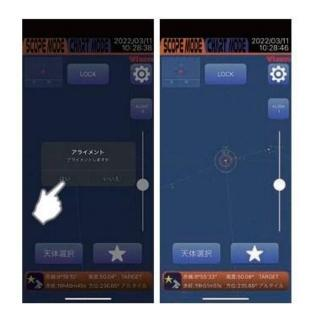
(6) It is necessary to choose several alignment stars to increase the pointing accuracy of your Go-To slewing. Repeat the procedures from (2) to (5) with different alignment stars. Aligning with stars of three or more will work practically.
