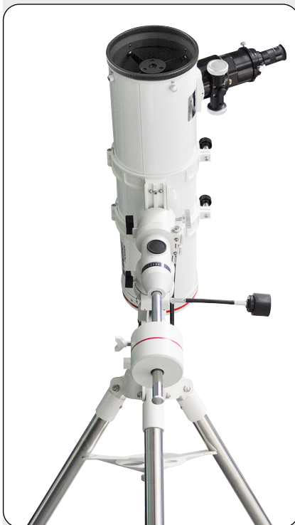
Fig. 16b: The parallactic home position seen from the north. The RA axis and the parallel tube point to the polar star (Polaris).
