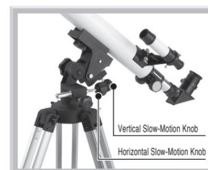
(Note) The slow-motion knobs turn within the limited range. If you want to turn them further, loosen the vertical / horizontal motion clamp and move them to the desired point and re-tighten the clamp. Then, adjust the direction with the slow-motion knobs.
