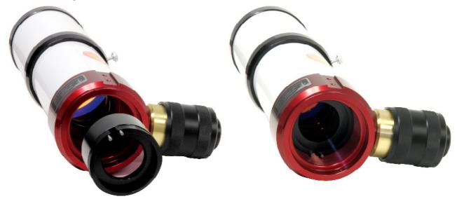
Remove the DSII double-stack module from your telescope. Now take the HRG anti-reflection filter and press the two silver knobs together that the HRG housing fits into the telescope. Move the HRG inside the telescope as far as it will go. Now you can again install your DSII module at the telescope, that's all. Now you can start solar observing.
