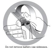
Do not remove battery cap sidewa Locking tabs could break.
