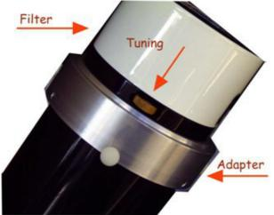
Slide the drawtube of the Lunt Solar Systems blocking filter into your focuser and tighten the retention system of your telescope.
