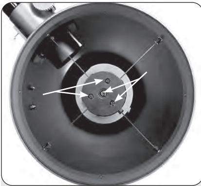
Fig. 31b: The four collimation screws in the secondary mirror housing
