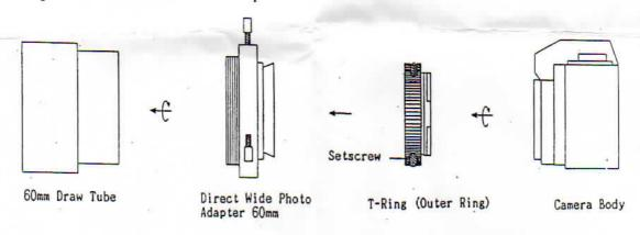
Attach the T-Ring to the Direct Wide Photo Adapter 60mm and lock it with the setscrews.
