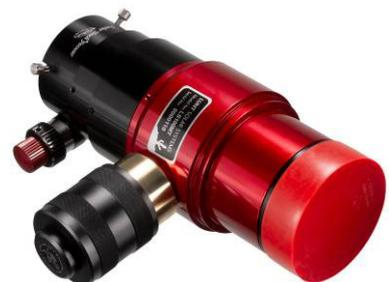
In this version without H-alpha unit the telescope can also be used for observing the sun in white light together with a Herschel-wedge, or together with a LUNT Ca-K module for observing the sun in the Ca-K wavelength:
