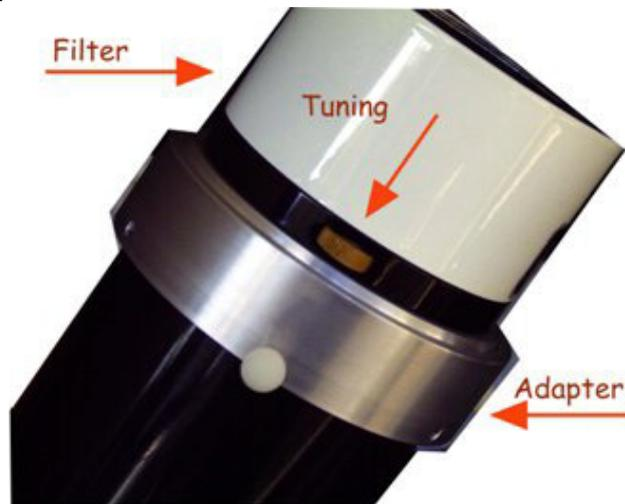
Slide the drawtube of the Lunt Solar Systems blocking filter into your focuser and tighten the retention system of your telescope.
