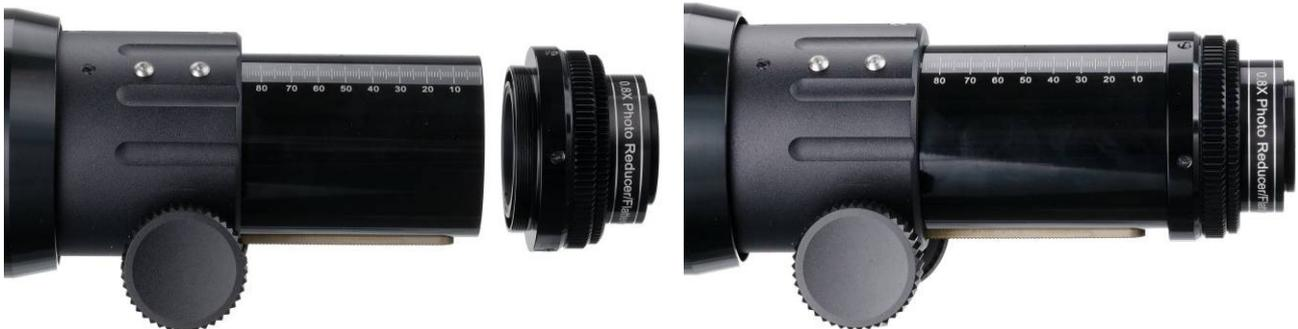
A DSLR camera with a suitable T2 adapter ring can now be connected directly to the upper side of the reducer/field-flattener. DSLR cameras and the corresponding T2 adapter rings are usually standardized, which means that the required working distance to the reducer/field flattener is automatically provided here.
