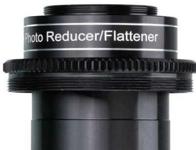
If other threads are required for connection to the telescope, the flat adapter ring can first be screwed onto the M54x0.75 thread of the reducer/field-flattener. Then an M68x1 male thread is provided on the telescope side.
