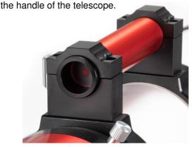
Look thru the eyepiece. Do you see a fuzzy red ball? If not, make sure you have removed the dust cap from the front. After some trial and error the Sun should appear in the eyepiece.
