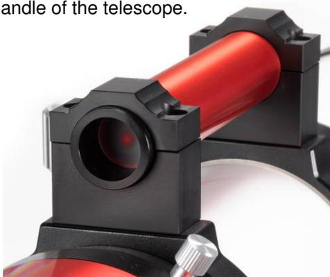
Look thru the eyepiece. Do you see a fuzzy red ball? If not, make sure you have removed the dust cap from the front. After some trial and error the Sun should appear in the eyepiece.
