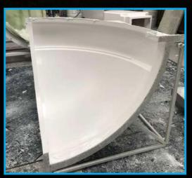
The moulds Pulsar use to fabricate the domes.
